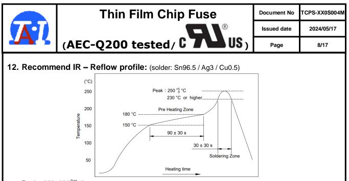
Peak :  $250+5/-0^{\circ}C$ , 5 sec. Pre-heat Zone : 150 to 180  $^{\circ}C$ , 90±30 sec Soldering Zone :  $230^{\circ}C$  or higher ,  $30\pm10$  sec
